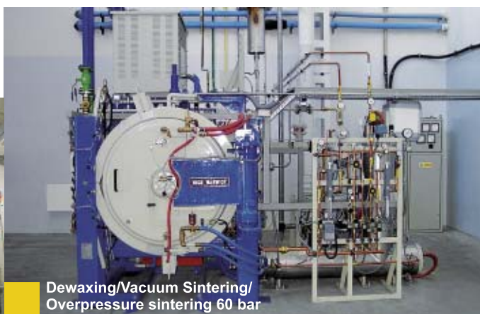
Vacuum purged, retrofit dewaxing-sintering for temperatures below 1000°C
