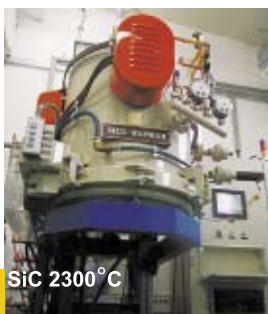
Dewaxing/Vacuum Sintering/ Overpressure sintering 60 bar
